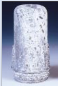
Rapid corrosion of untreated aluminium.
