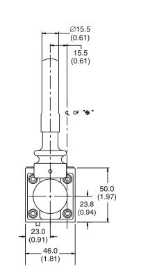
Note: 22.0 mm (0.87") from bottom of bolt hole counterbore to bottom of valve.
